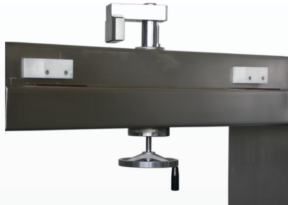
clamp system equipped with manual swivel clamp
