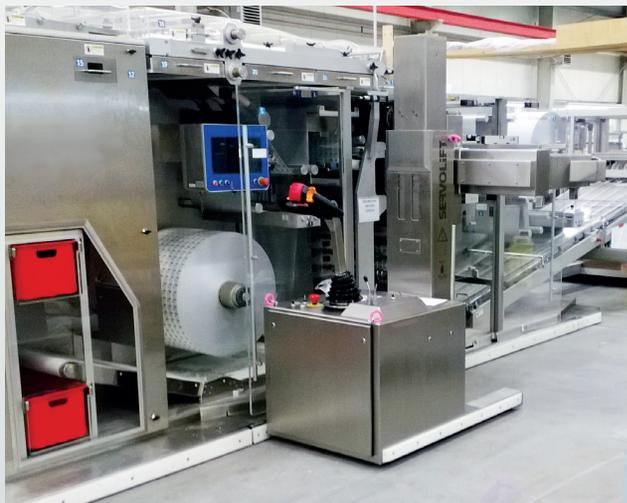
Sideways positioning at the packaging line for exchange of the foil reel
